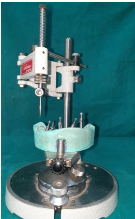
Figure 2. Surveying of cast with impression post.
